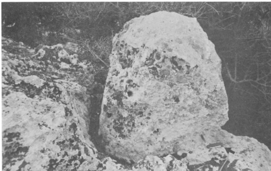
Figure 3. Block partially separated by Method 1, Figure 1, in Son Carla quarry. Jackknife, indicated by arrow, gives scale and lies in the mechanically cut trench.
